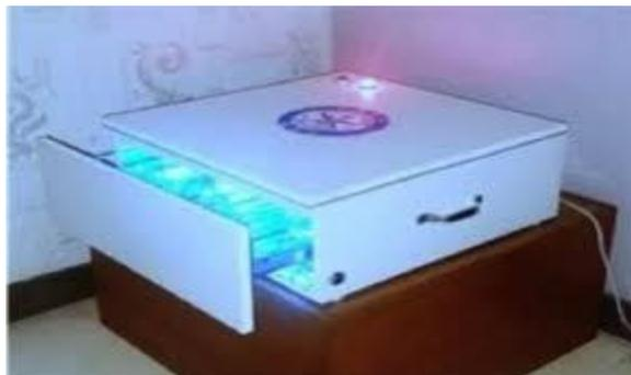
On May 10, 2020, Research Centre Imarat (RCI), Hyderabad based Defence Research and Development Organization (DRDO) premier lab, developed an automated contactless Ultraviolet C (UVC) sanitisation cabinet called **Defence Research Ultraviolet Sanitiser (DRUVS)**. It has been designed to sanitise mobile phones, iPads, laptops, currency notes, cheque leafs, challans, passbooks, paper, envelopes, etc.
