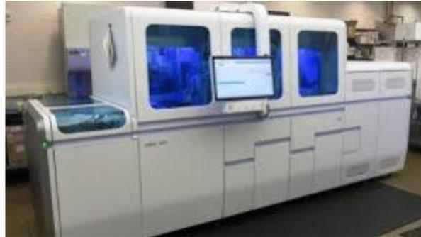
The COBAS 6800 is a fully automated, high-end machine for performing Reverse transcription polymerase chain reaction (RT-PCR) tests for COVID-19. The machine has been placed at the National Centre for Disease Control (NCDC) because it requires a minimum BSL2+ (Biosafety Level Two Plus) containment level for testing, and cannot be placed at just any facility.
